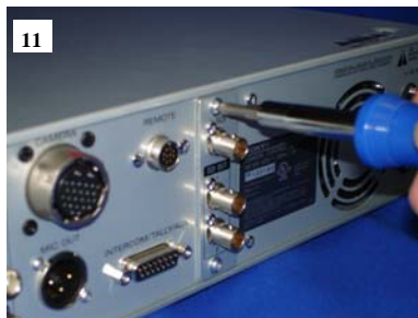
11 Reinstall the SDI card back into the CCU and tighten both screws to secure.
