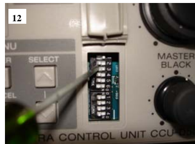
12 On the front of the CCU-D50 make sure you change the dip switch #3 to the ON position to enable Digital Transmission
