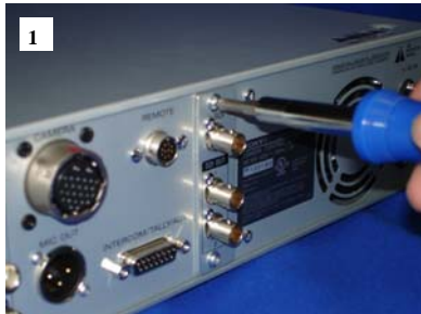
1 Remove the two screws from the SDI card located on the rear panel of the CCU-D50
